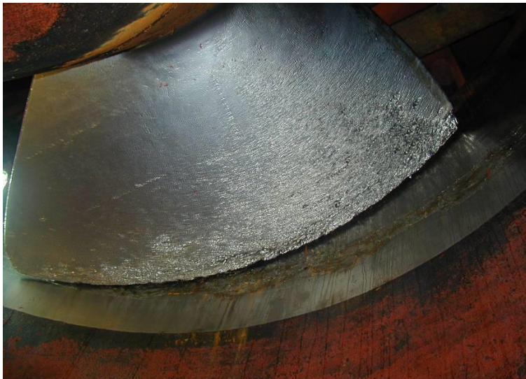
Uncoated and damaged runner
